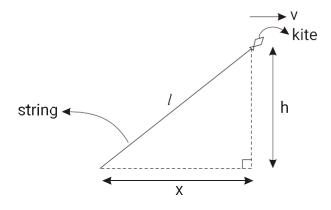
Let at any moment, the length of the string be 1. Then by Pythagoras' Theorem, we get,  $I^2 = x^2 + h^2$ . Differentiating both sides with respect to time, we get,  $\frac{dl}{dt} = 2x \frac{dx}{dt} + 0$ . (The height h of the kite above the ground is constant)
