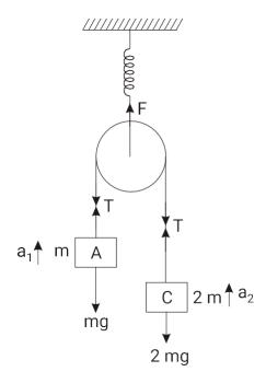
The spring force does not change instantly. Just after cutting the string, the spring force will be 4mg. Since the pulley is massless, the net force on it is zero even when it is moving. So, the tension tension in the string passing over the pulley is still 2mg.
