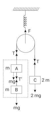
The masses on both the sides of the pulley are the same. So, the system is in equilibrium. From the equilibrium of C, T = 2mg.
