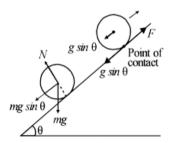
When cylinder rolls up the incline angular velocity decreases for that torque of friction should be in opposite direction of angular velocity . Therefore friction must be acting up the incline
