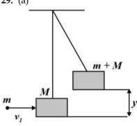
As block raises to a height y, therefore speed just after collisions is  $v_1 = \sqrt{2gy}$
