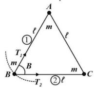
Massless rod l can exert force  $T_1$  and B only along its length i.e., towards the centre of the circular path. Hence  $T_1$  contributes only to centripetal acceleration of B.
