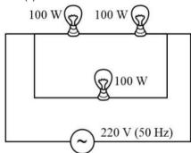
For the two bulbs in series, equivalent power is
