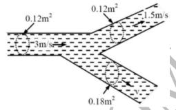
From equation of continuity  $Av = A_1v_1 + A_2v_2$
