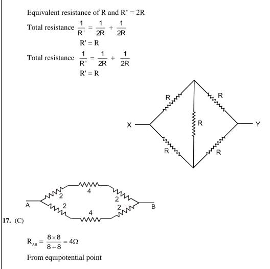
18. (c)The equivalent resistance of the circuit
