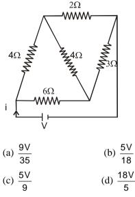
24. The total power dissipated in watts in the circuit shown here is :-
